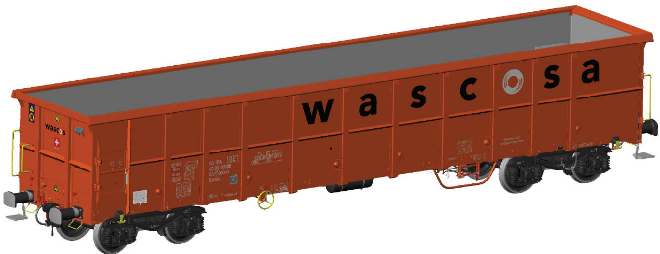
Four-axle open wagon (standard wagon), Eanos, 82.5m 3 - angle view
