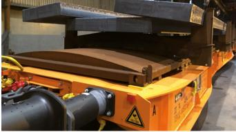
The Wascosa flex freight system® in use with superstructures for steel transport and rail infrastructure construction.
