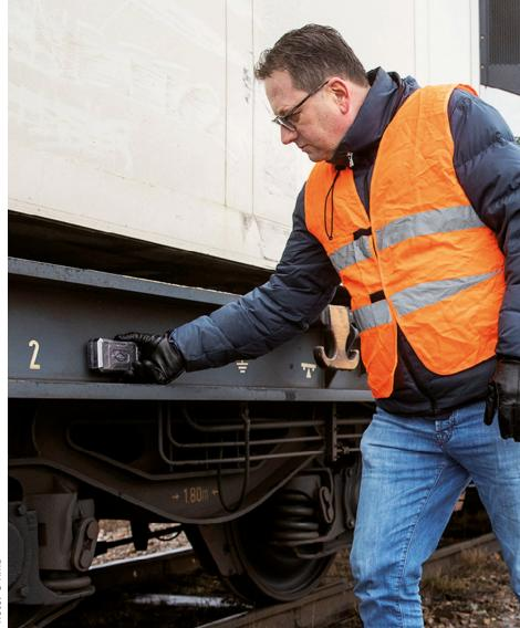
${\it The RMD performance monitoring device installed on an intermodal wagon.}$
