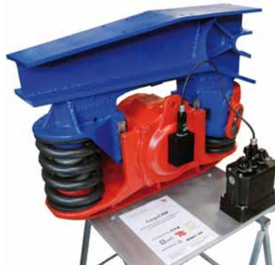
Model of data collection on the axle bearing cover and data transmission to the processing and storage box
