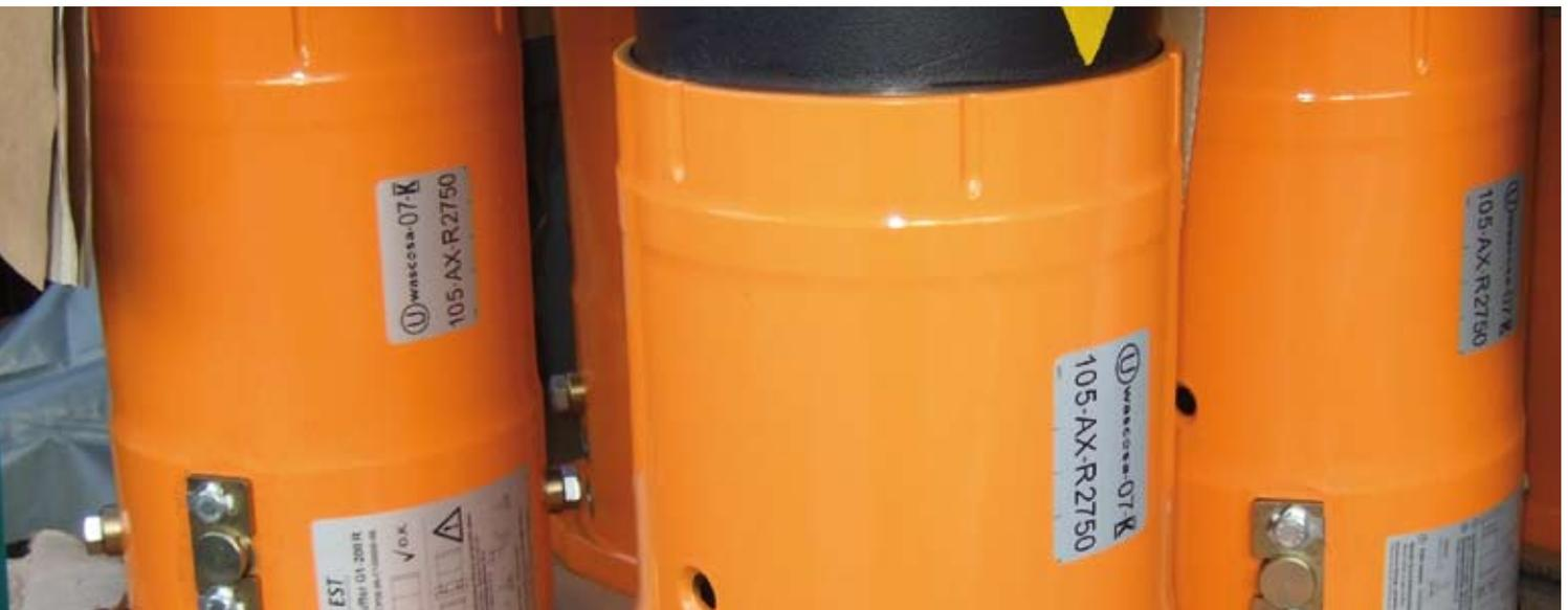
Standard components will be freely exchanged in future in the Cargo Rail Service Center CRSC, e.g. crash buffers for retrofitting hazardous goods cars according to RID (see article on page 10).
