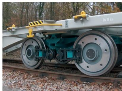
New technical solutions are required for a new track price system. JOSEF MEYER Transport Technology AG provides this with its pivoted bogie LEILA. The design of the light and low-noise freight traffic bogie LEILA is distinguished by
