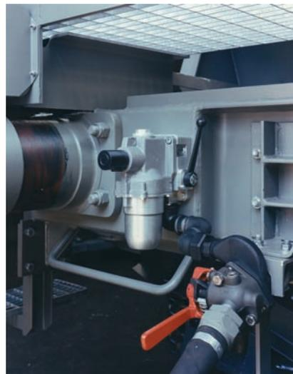
*Derauling detectors are fitted to buffer beam at each end of the car and are pneumatically connected to the train's main air line via a 1"-line.*
