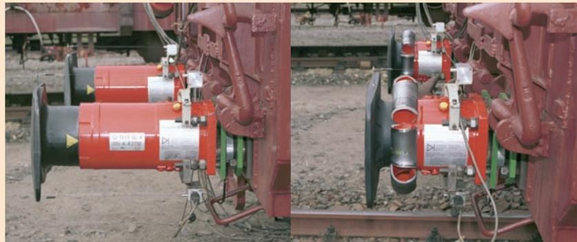
Example of a crash buffer before and after deformation.
