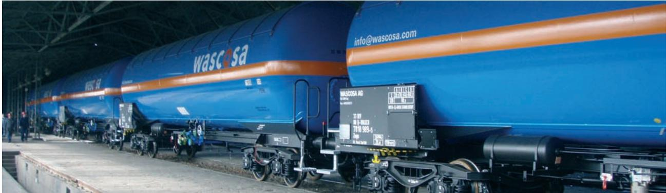
Pressurized gas tank cars are identified by the orange warning stripe around the tank and are used for various gases. A differentiation is made between the following gases:
