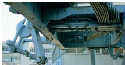
The push-and-pull device from the year 1928 is very similar to the materials still used today. The particular aspect of the pulling device is that it was built on the basis of leaf bearing springs.
