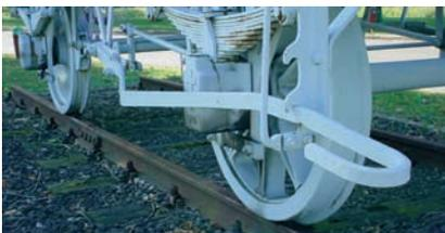
There are no compressed-air brakes. During operation, it was not possible to brake the individual car. For this, it has a securing brake that was only used for parking. The original spoked wheelset is from the KRUPP company. The second wheelset from 1905 was supplied by the company HB&HV.
