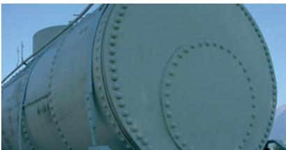
The entire tank car has been processed with head-rivets from dome to undercarriage. The tank itself is situated on a wooden base and is held only by strap retainers. As a result, no saddle sheets were required.
