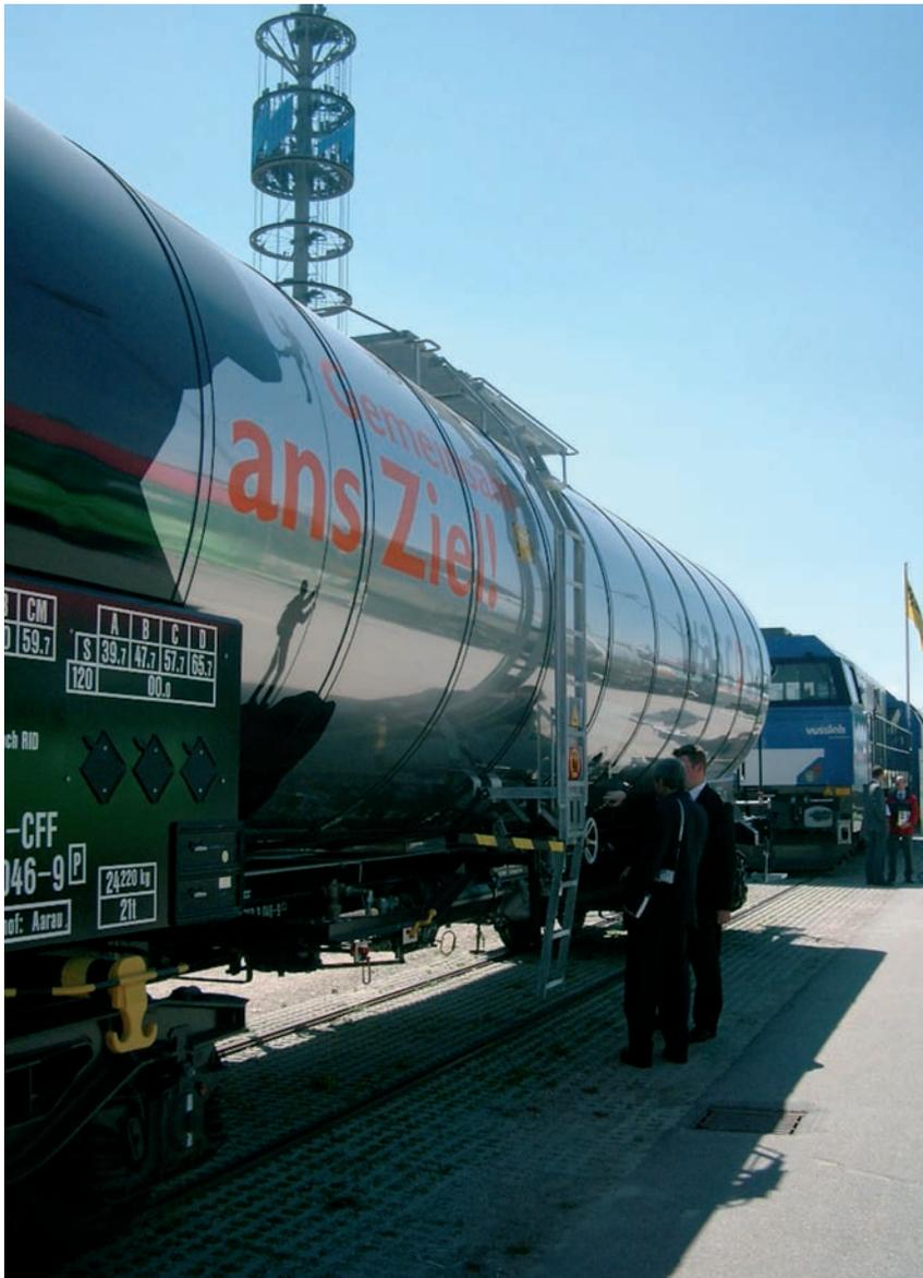
*The eye-catcher in the open-air section – chemical tank car for transporting caprolactam.*
