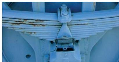
The truck's suspension was ensured through 11-layer leaf bearing springs. An interesting aspect is that it was also possible to re-lubricate the wheelset bearings individually. A re-lubrication cover was attached to the wheelset bearing for this purpose. You can no doubt still recall the men with their traditional oil cans.
