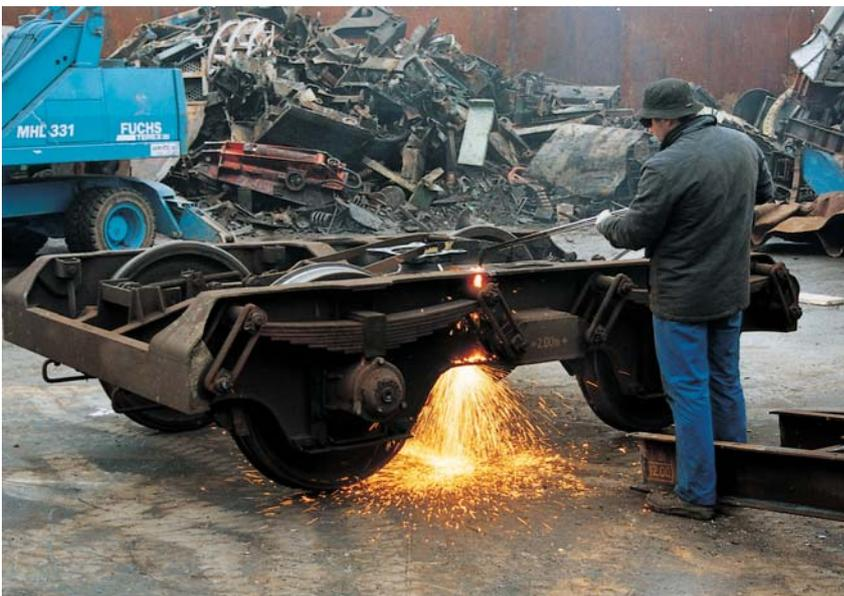
*Recuperating is manual work: worker welding a bogie.*
