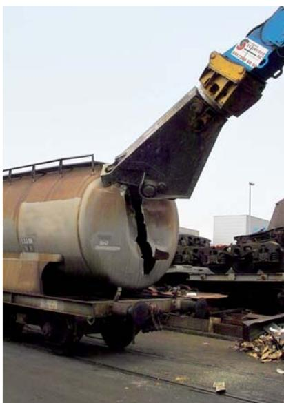
*Heavy machinery for scrapping tank cars: scrap shears in use.*
